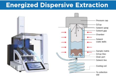
Q-Cup Technology combines the processes of Pressurized Fluid Extraction and Dispersive Solid Phase Extraction into one instrument.
