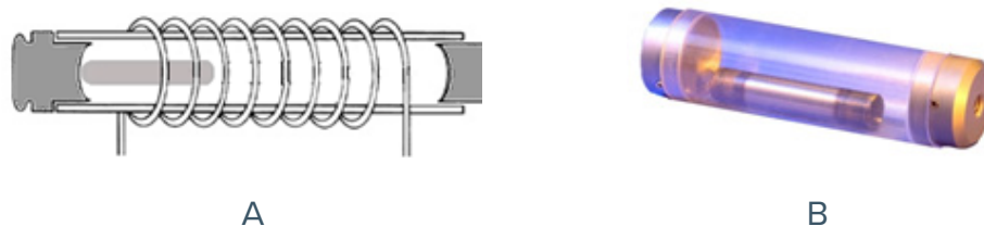
Figure 3. Illustrations of (a) cross-section of solenoid magnetic impact mill and (b) grinding container (Spex SamplePrep)
