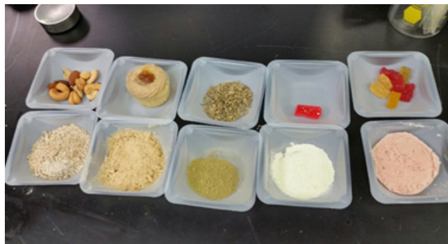
Example: Before and after results using the Spex SamplePrep Freezer/Mill ® for several representative matrices commonly encountered with regard to infused/edible products
