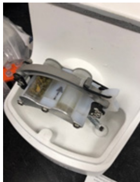
Example: GenoLyte ® configured for 2 x 7 mL tubes loaded with 0.5 gram of cannabis (hemp)
